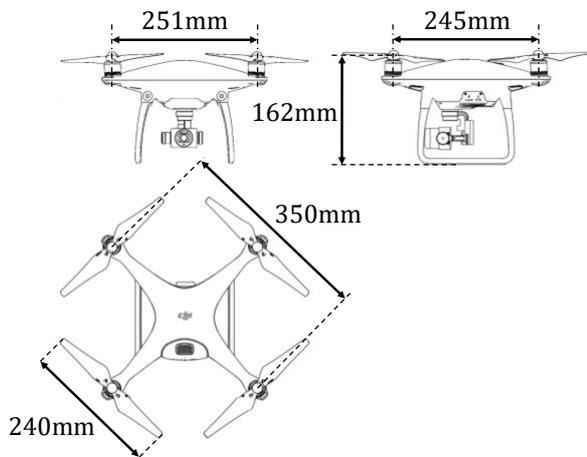
Fig.10 : Phantom4 measurement
