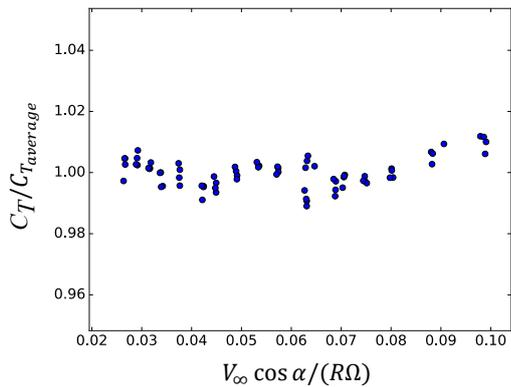
Fig.8 : the fluctuation value of measured  $C_T$  in this experiment [3]
