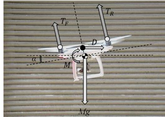
Fig.9 : Force and moment at forward flight
