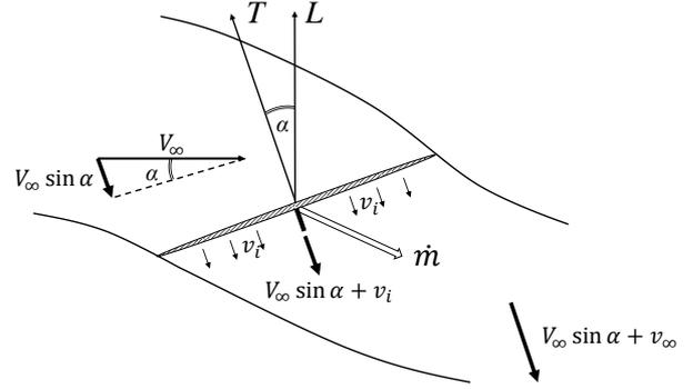
Fig.4 : A change of the momentum in forward flight
