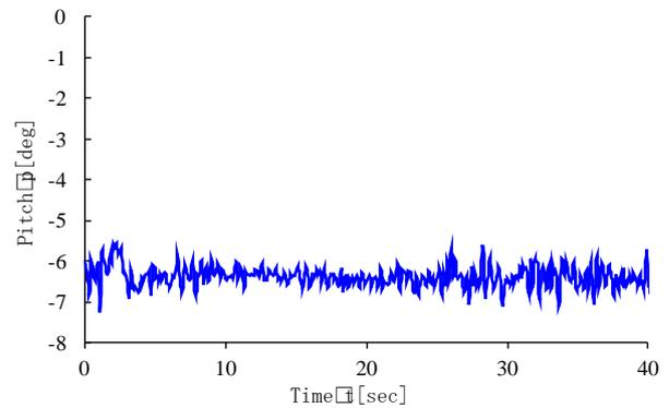
Fig.7 : An example of steady flight data(pitch angle)
