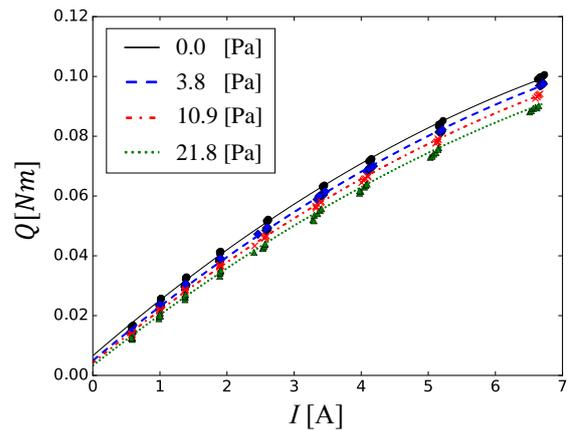
Fig.3 : The relationship between current  $I$  and torque  $Q$  at each dynamic pressure.
